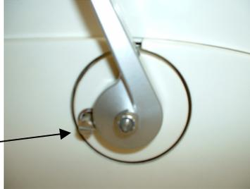
5. Once tape is properly loaded and the brush and water tank are in place, you are ready to dispense the tape. With the adjustable feed stop set at your desired length, simply pull the handle downward and the tape will be dispensed and cut.
